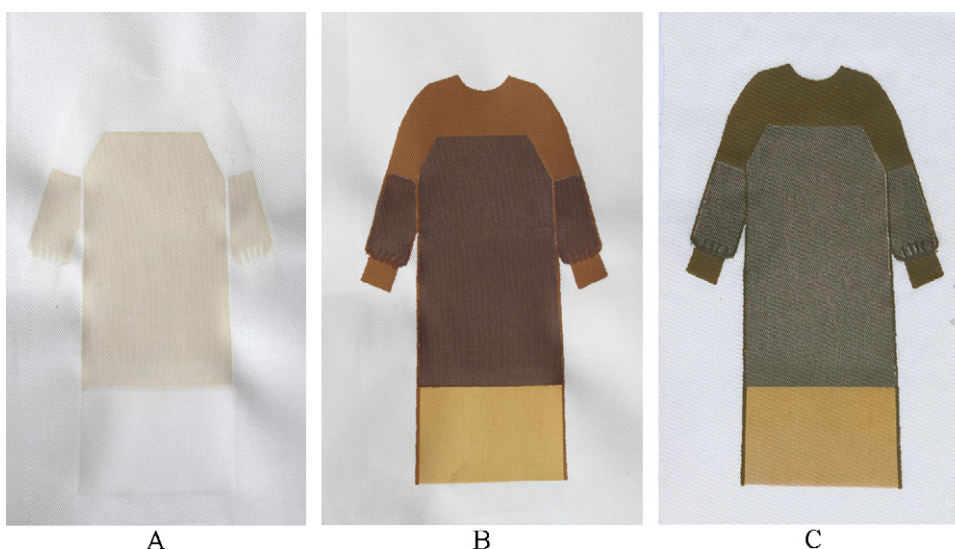
Fig. 6. Photographs of example protective uniform: (A) a cotton cloth after printing; (B) the same cloth after UVC irradiation (absorbed dose equaled to 5 \text{ J/cm}^2 ); and (C) after one washing. (For interpretation of the references to color in text, the reader is referred to the web version of the article.)
